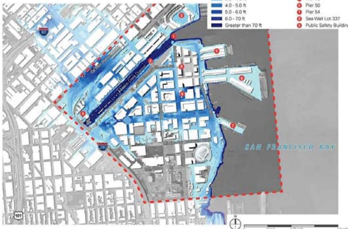
2050 inundation level projection, sea level rise adaptation study for Mission Creek, San Francisco
